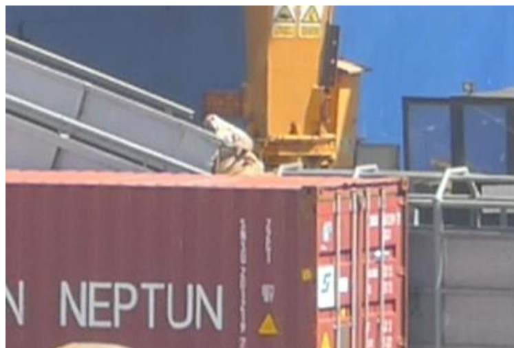
Figure 37. Dangerous gap at the beginning of the ramp posing risk of injuries. We saw animals' heads getting stuck there during hasty loading.
