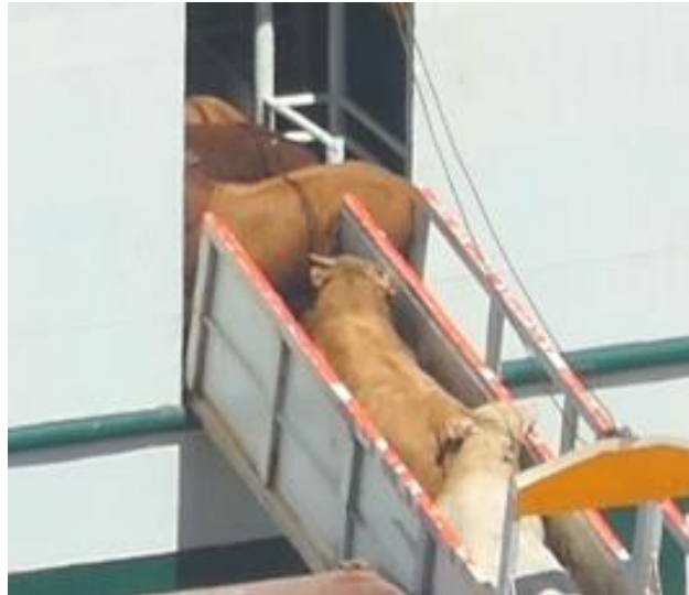
Figure 30. Gap between loading ramp and vessel with potential risk of injuries.
