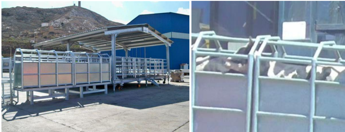
Figure 2. Movable gangways between the solid corridors and the movable ramps from the vessel. Due to their construction, the movable gangways pose a risk of injuries, especially for the animals with long horns. We observed several animals with horns stuck between the metal bars. Cartagena Port, 08/06/18.
